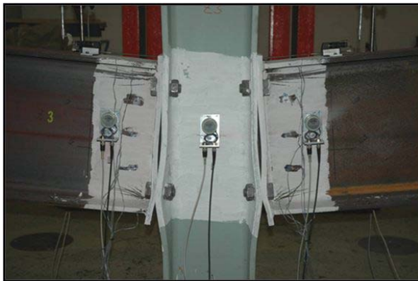
Figure 9: Ductile tension components of bolted beam-to-column-connection
