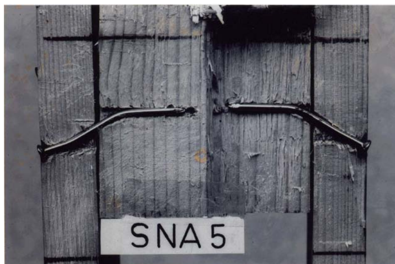
Figure 7: Opened nailed connection after a test to determine the load-carrying capacity in shear. Blass (2003)
