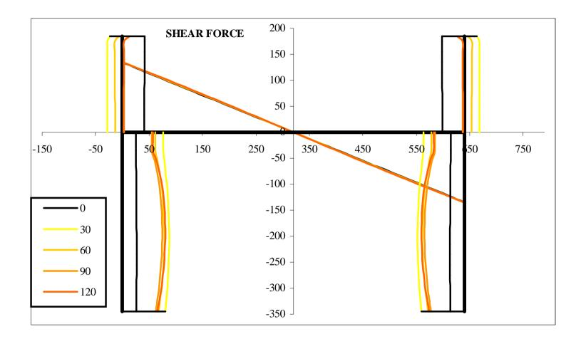
Shear force in lower columns x 4 -> danger of shear failure (detailing according to seismic provisions?)
